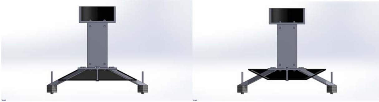
Figure 8. Section views showing internal bolt for ballast and bottom plates
