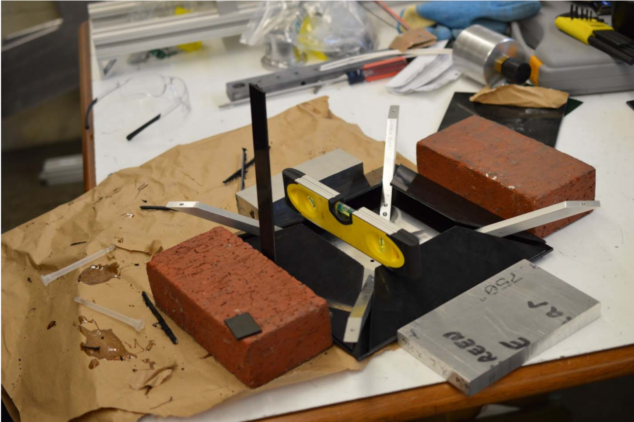
Bracing the inverted skirts in place while the epoxy sets
